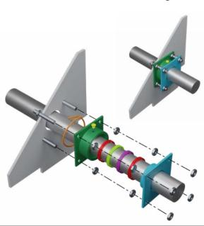
Theory of Operation — The stuffing box is sealed to the fan housing with PTFE joint sealant for a gasketing material. The packing materials are a flexible graphite split ring and a lantern ring sandwiched between two carbon yarn anti-extrusion rings. The outside hex nuts force the outside packing plate into the stuffing box, expanding the graphite rings to provide a leak tight seal. A pressure purge tap is provided to insure that all leakage will be the purge gas.
