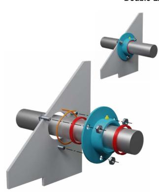
**Theory of Operation** — The sealing action is provided by two lip type seals placed back to front within a seal housing with a layer of grease between them. The grease reservoir may be maintained using the grease fitting in the seal housing. The contact is between the seal inner lip and the circumference of the fan shaft.
