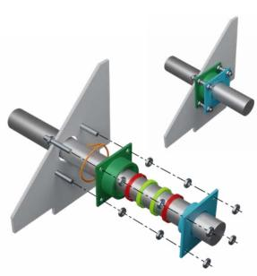
Theory of Operation — The stuffing box is sealed to the fan housing with PTFE joint sealant for a gasketing material. The packing materials are two flexible graphite split rings sandwiched between two carbon yarn anti-extrusion rings. The outside hex nuts force the outside packing plate into the stuffing box, expanding the graphite rings to provide a leak tight seal.
