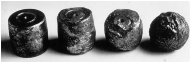
Figure 9. Damaged Spherical Bearing Rollers
