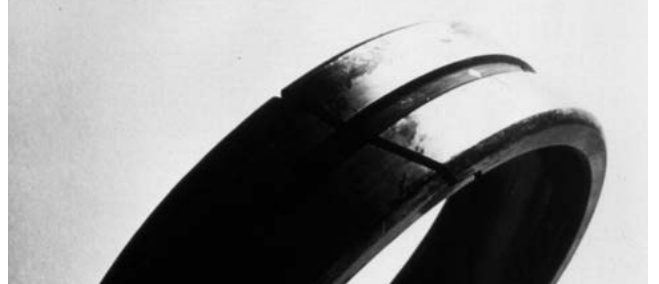
Figure 26. Pits Caused by Electrical Current
