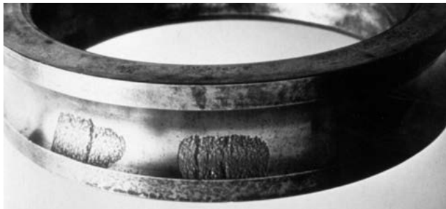
Figure 21. Two Load Zones on the Outer Race
