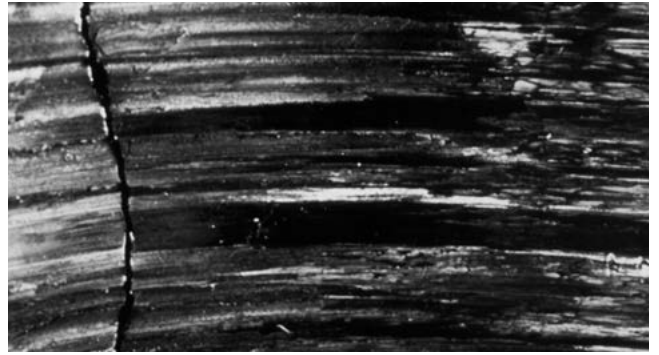
Figure 23. Fretting Corrosion on Bearing Bore
