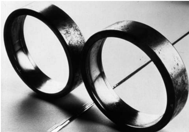
Figure 21. Two Load Zones on the Outer Race
