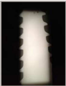
X-RAY OF HOLDING PATTERN (OLD SHAFT)
