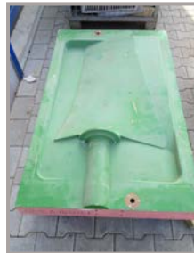
CASTING MOLD FOR REPLACEMENT BLADE
