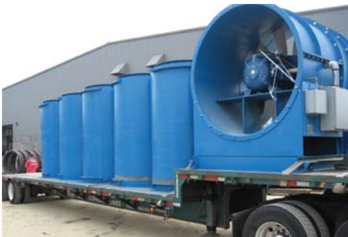
Partial shipment for the LA Metro contract that included eight 2M central fans and eight 1.25M jet fans.
