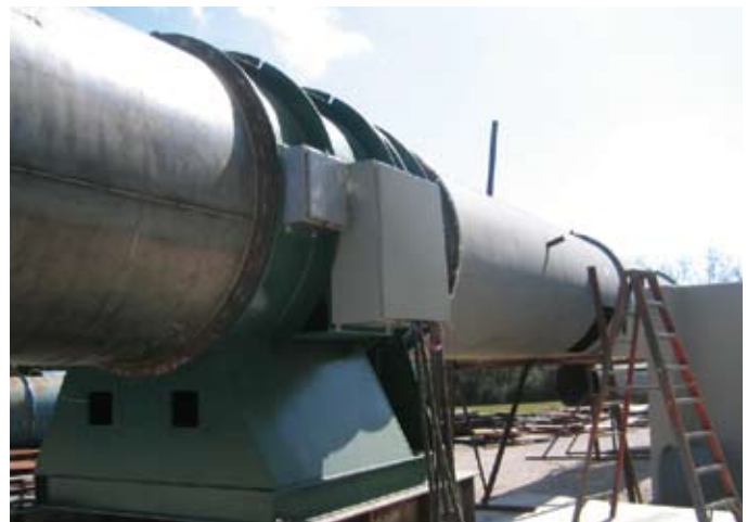
A NYCT axial fan set up on an AMCA 210 test stand.
