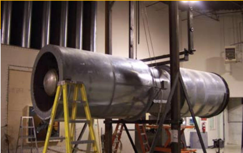
Picture shows a standard AMCA 250 suspended thrust test for a jet fan for the City of Atlanta Archer Western contract. Clarage will also complete this test on a thrust table for larger units.
